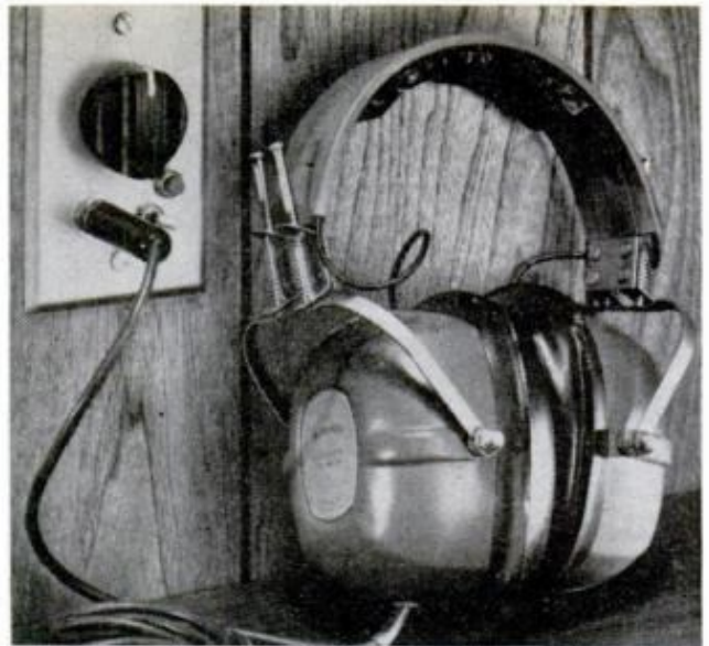
into a standard wall box, it contains a dual L-pad volume control, stereo phone jack and a low-voltage pushbutton switch to turn hi-fi power on and off
